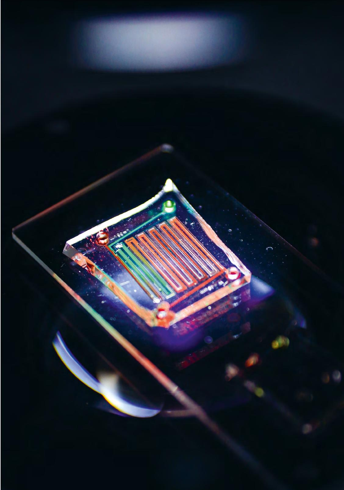
Fascinating view of the microchannels on a microfluidic chip. This chip, no larger than a coin, features microscopic channels through which fluids can circulate in a highly precise manner. In the search for cancer therapies, this technology makes it possible to perform high throughput screening of cancerous cells encased in micro-droplets, opening up countless new opportunities for biomedical research.
